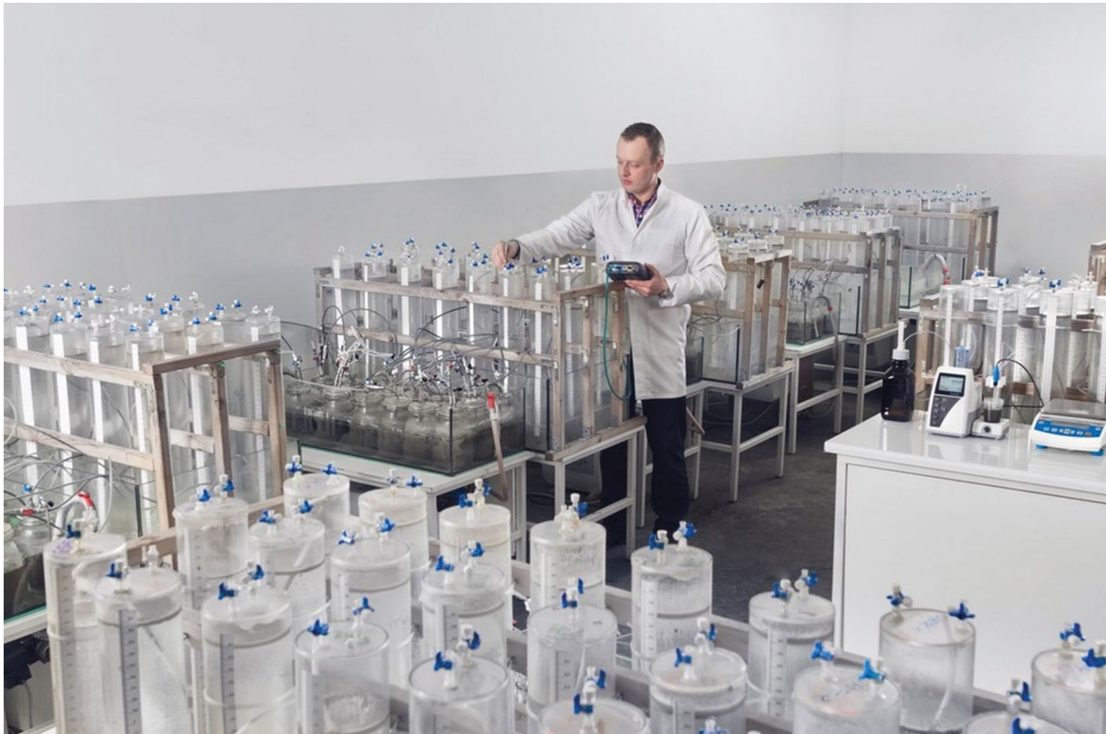
FIG. 17. Biogas/methane efficiency test reactors according to DIN 38 414/S8
